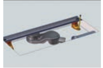
Kanalı teraziye alarak zeminden işaretleyiniz. Adjust height adjusting set with scale according to the ground level.
