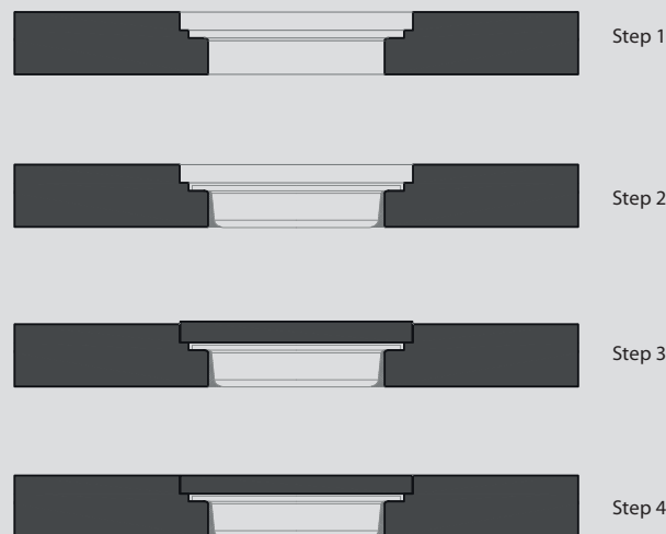
Detail of the anchor sleeve on the KRION tubular profile
